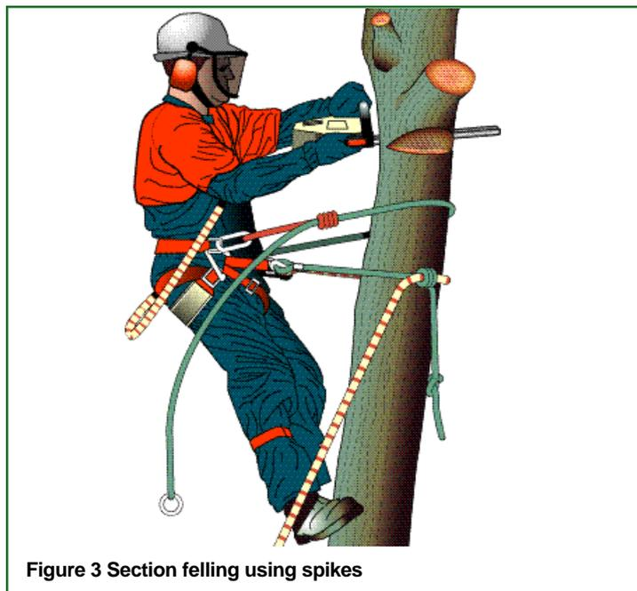
Figure 3 Section felling using spikes
