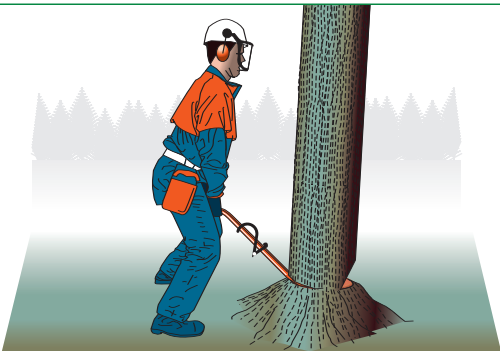
Figure 3 Use of breaking bar
